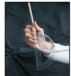
Fig. 3: Dual pointer with affixed protractor.
