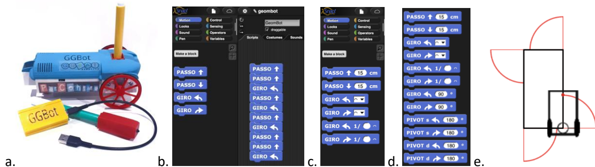
Figure 16: a) GGBot with a marker placed in its posterior holder; b) initial command set and example of code; c, d) commands with parameters for more advanced programming; e) drawing made by the virtual GGBot given the code in b)
