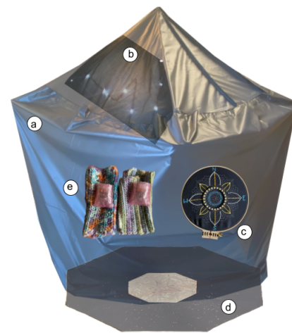
Figure 2: STARR components: (a) Planetarium; (b) LED constellation; (c) hand-held compass; (d) Octagonal rug; and (e) Mugic glove sensors.
