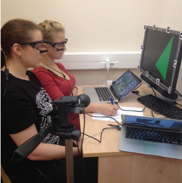
FIGURE 6.3 Dual eye-tracking experimental setting where two participants discuss an image on a shared screen
